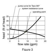
To find the flow rate through the circulator draw a line straight down from the intersection of the curves to the lower axis of the graph. To determine the differential pressure across the circulator draw a horizontal line from the operating point to the vertical axis and read the head added to the fluid as it passes through the circulator. Then convert that head number to a corresponding differential pressure using Formula 1.
