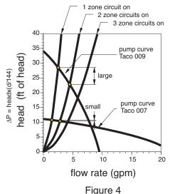
Using a circulator with a flat pump curve in zone valve systems is not a new concept. It's been described in many references over several decades. Still, some installers have the mistaken impression
