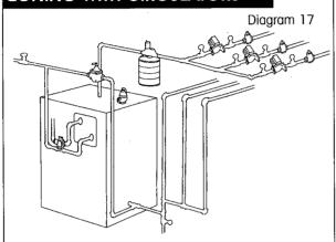
In residential systems using circulators with less than 12 feet of shutoff head, circulator location is not critical. However in a commercial system, it is always best to pump away from the boiler and expansion tank.
