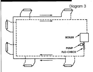
In this system, the first terminal heat transfer unit (in relation to the boiler) taken off the supply main is the last one connected to the return main. Conversely, the last unit of the supply is the first connected to the return. Since the length of flow path is the same for each terminal heat transfer unit, the two-pipe, reverse return system provides a uniform flow and each terminal unit receives its proper share of water.
