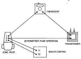
The wiring diagram for additional TACO zone valves with an intermittent pump is shown in diagram 13.
