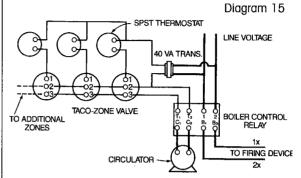
TACO-ZONE WIRING DIAGRAM SHOWING TRIPLE FUNCTION HIGH & LOW LIMIT, CIRCULATORS & BURNER CONTROL RELAY FOR FORCED HOT WATER HEAT WITH DOMISTIC HOT WATER. GAS OR OIL FIRED BOILERS.
