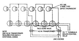
NOTE EACH TACO-ZONE VALVE IS RATED AT 0.9 AMPS AT 24 VOLTS. A MAX OF 3 VALVES REPRESENTS AN INTERMITTENT LOAD WHICH CAN BE ADEQUATELT CARRIED BY ONE 40 VA CONT. DUTY TRANSFORMER
