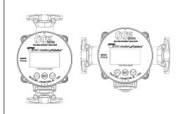
Position electrical knockout at 6 o'clock position for best programming and LCD viewing orientation.
