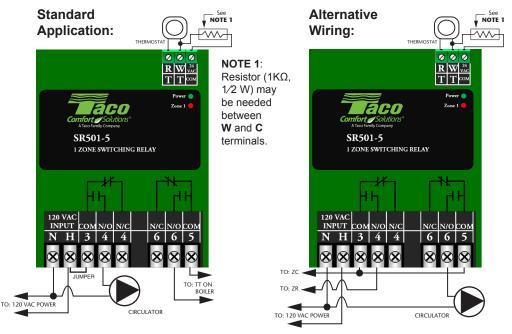
**NOTE 2:** When using Alternative Wiring diagram, the boiler operating control's ZC terminal will see the load of the circulator(s).
