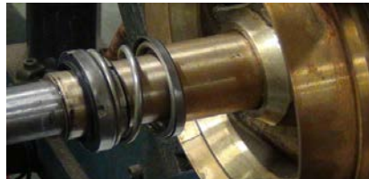
Mechanical Seal Assembly on Sleeve
