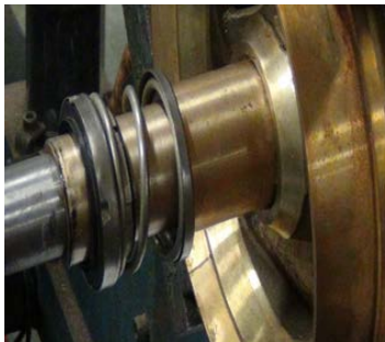
Removal of Mechanical Seal
