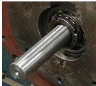
Bearing Retainer Nut and Lock Washer
