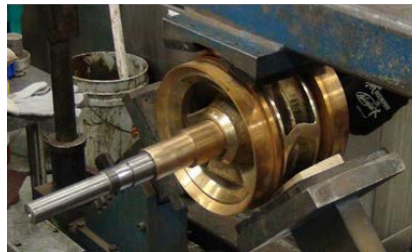
Sleeves on Impeller Shafts with Concealed O-rings
