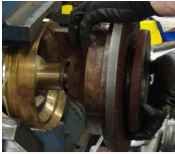
Removal of Bearing House and Bearing Cap
