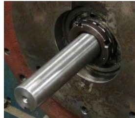
Bearing Retainer Nut against Lock Washer
