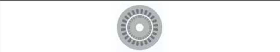
Fig. 1.29 Rotor with pole gaps on the circumference placed in the stator
