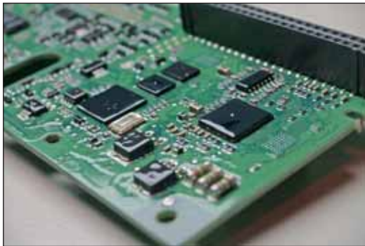
Fig. 9.8 Printed circuit board with conformal coated
