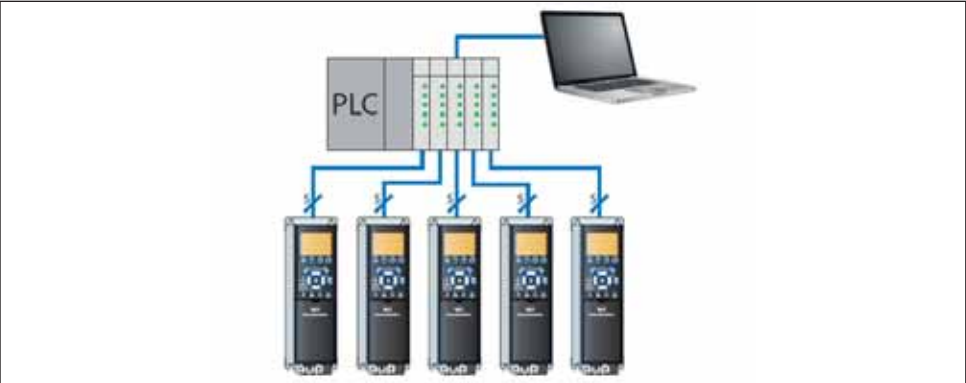
Fig. 8.7 Traditional wiring. No fieldbus
