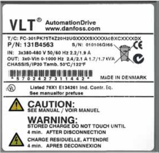
Fig 9.2 Identification data of a Danfoss frequency converter
