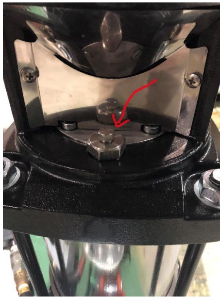
Figure 3: Bleed Valve of a VR Pump
