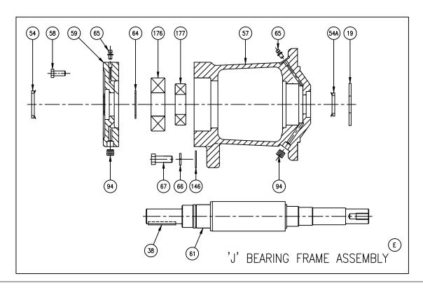
NOTE: Note difference in visual appearance of bearing frames on pages 2 and 3. New frames are a direct replacement for older ones. The part numbers for individual bearings are different from old frames to new frames. If you need help determining which frame you have, please contact tech services at Taco (401-942-8000).
