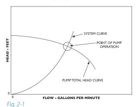
Care must be taken that both pump head and friction are expressed in feet and that both are plotted on the same graph. The system curve will intersect the pump performance curve at the flow rate of the pump because this is the point at which the pump head is equal to the required system head for the same flow.
