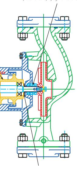
Replaceable corrosion resistant shaft sleeve incorporates a "built in" slinger to deflect water away from the bearing cartridge in the event of a seal leak.
