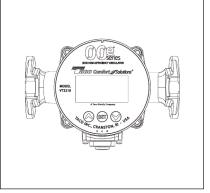
Position electrical knockout at 6 o'clock position for best programming and LCD viewing orientation. Casing may be rotated to change flow direction.
