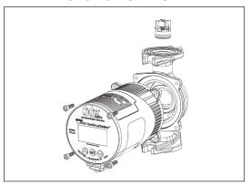
To rotate the casing, remove the 4 motor screws and spin the casing to the desired flow direction. Reattach the 4 screws  $\{\%_{32}^{\rm u}$  allens wrench required). Be sure body gasket is seated evenly to prevent leakage. Tighten motor screws to 34-42 inlbs torque.
