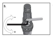
3. Using the wrench to support thelocking nut and prevent it from rotating, turn the Allen key to adjust the outlet temperature clockwise to decrease the temperature, counterclockwise to increase the temperature - until the desired set point is reached.
