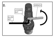
2. Holding the 3/16" Allen key (supplied), loosen the locking nut with a 7/16" wrench.
