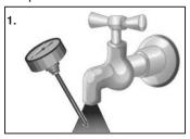
Using an accurate thermometer, test the mixed water temperature at the nearest outlet being supplied by the valve. The test outlet should not be a shower with its own temperature limiting control valve. This should be opened to allow a minimum flow rate of 1.5 gpm (6 L/min). Allow the water to run for at least one minute to ensure the mixed water temperature has settled.
