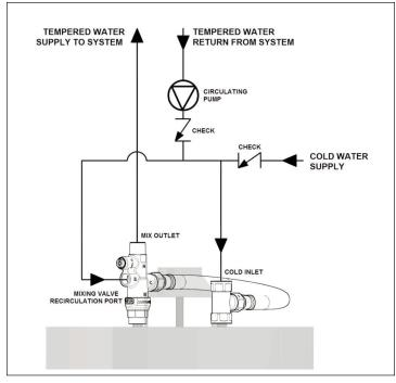
**NOTE:** This diagram is a guideline only. Any installation of a recirculated system should be undertaken by a qualified tradesman, and in accordance with the relevant codes and State, Provincial and Local Authority requirements. Performance of the system will be dependent on the other components specified within it.
