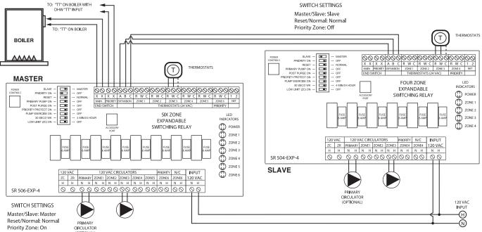
Replacement Switching Relay fuses part number: SR6A-001RP (Manufacture: Littlefuse, Part Number: 229006)
