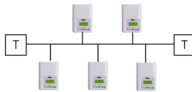
Figure 3.2 Doubly Terminated Bus Topology
