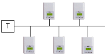
Figure 3.1 Singly Terminated Bus Topology
