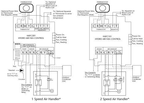
\* Both HAFC101 and 201 capable of 1 and 2 speed applications
