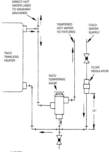
NOTE: INSTALL TEMPERING VALVE BELOW COLD WATER INLET TO HEATER
