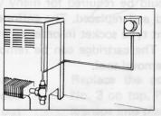
5. CONVECTOR OR ENCLOSURE Wall mount dial mounted away from heat influence of radiator on a nearby wall or actually on convector cover if provision is made to insulate sensor from heat influence of cover.
