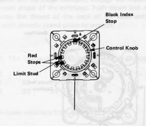
Remove red stops from their stored locations and place them in slots on the Control Knob, one on each side of the Limit Stud.
