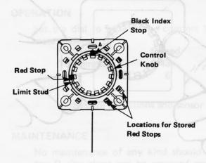
Remove a red stop from its stored location and place it in the slot of the control knob just above the limit stud.
