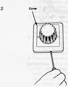
Pry cover off by inserting a tool at the small oval hole in the bottom of the cover.
