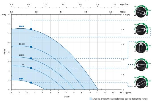
3 fixed speed settings ( $\triangle$ ) (Low, Medium High) allows the installer to choose the speed and flow rate to precisely match system requirements. It also has infinitely variable speed settings between MIN/MAX to fine tune flows more precisely. Pre-marked 003/006 settings enable installers to set 006e3 to match standard 003 or 006 performance.
