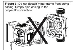
To rotate the pump casing, remove the 4 motor screws using a 5/32" (4 mm) allens wrench. When rotating pump casing position, DO NOT detach motor housing from the casing. Damage to the casing O-ring and leakage may result. Simply spin casing to the proper flow direction desired as shown in Figure 4 and Figure 5. Reattach the 4 screws. Be sure motor is positioned correctly and is seated evenly to prevent leakage or damage to O-ring. Tighten motor screws evenly to 25-33 in-lbs torque.
