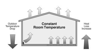
The heat supplied to the building is directly proportional to the temperature of the water and the surface area of the heating element. The higher the temperature of the water flowing through the heating terminal, the higher the heat output.
