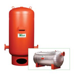
Capacity: 50–3,000 gal. (190–11,356 L) Connection Sizes: 2"–12" Standard Working Pressure: 125PSI\* Max. Operating Temp: 375°F † Available with a wide range of standard insulation packages. Larger sizes available
